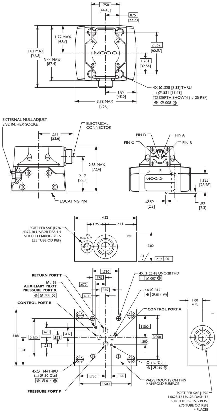
The mounting manifold must conform to ISO 10372-04-04-0-92. Surface to which valve is mounted requires a  $\sqrt{32}$  [ΔΔ] finish, flat within 0.001 [0.03] TIR.
